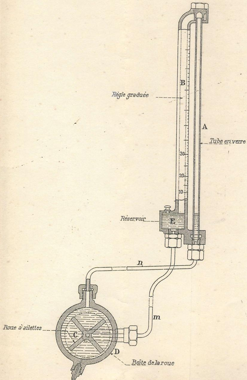
CHRONOTACHYMÈTRE ET PRISE DE MOUVEMENT
