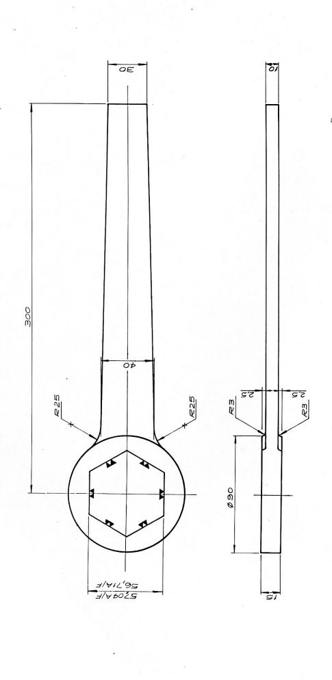
Spanner for bursting disc filting see 515 1016
