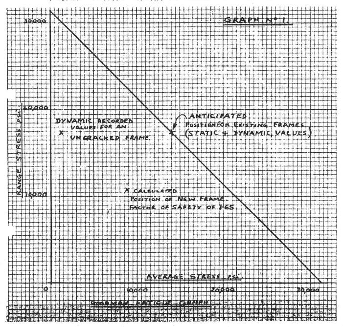
Now THESE FRAMES Do CRACK, . . THE STATIC STRESSES" FROM THE WT. OF THE BOILER MUST INCREASE THE AVERAGE STRESS BY AT LEAST 14,000 - 1260
