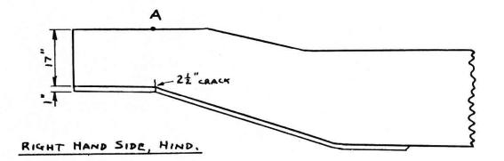
EXISTING FRAME. EFFECTIVE DEPTH OF CRACKED FRAME = 18"- 21" = 15.5"
