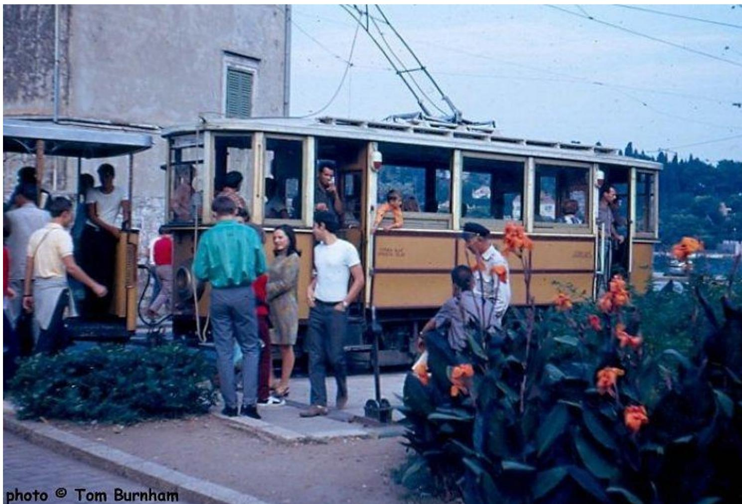
**Tom Burnham writes: a small system of 760mm gauge, with a Y-shaped layout - this is at the junction (see point lever in front of the tram). There were two versions of the 4-wheeled trams, one with a slightly more modern styling, running in motor-trailer sets. The afternoons tended to see power cuts, and the trams would regularly come to a dead stop along the Put Marsala Tita.**
