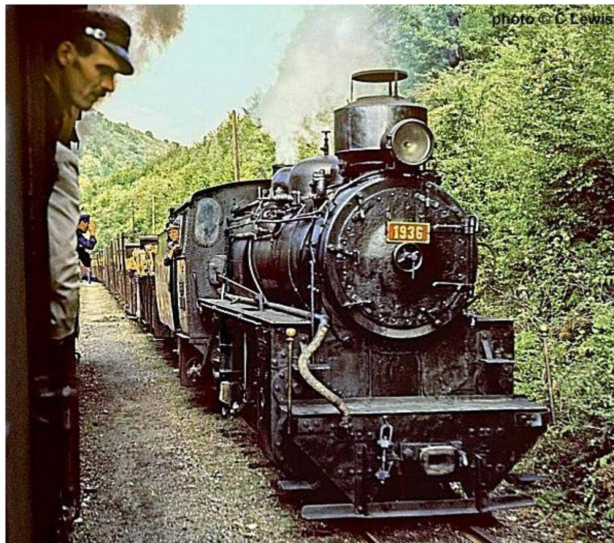
**The Czech firm of Skoda built a series of large 0-10-0's Nos. 1932 to 1937 in 1946. At least three of these impressive locos were working on the Steinbeis in 1965. This is No. 1936 which we passed at a loop between Prijedor and Drvar. No. 1937 is preserved in Doboj. Notice the salute of the passing train, saluting of trains and other staff members was a serious business back in 1965!**
