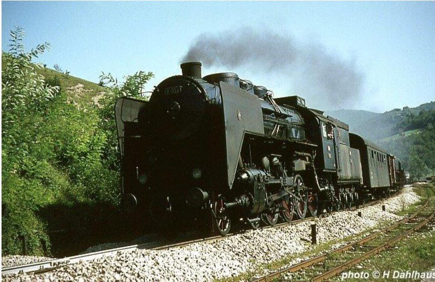
**With the 76cm line on the right this is 4-8-0 11-054 (MAVAG 7413/1955) with a goods train from Sarajevo at Semizovac on 11th August 1966. These impressive locos were identical to the Hungarian class 424 and a total of 63 were built for service in Yugoslavia.**
