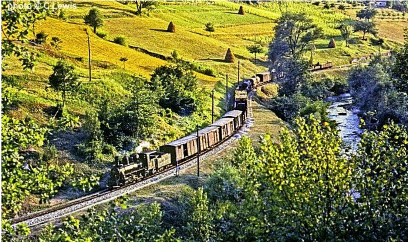
**The 73-class 2-6-2s could be fast locomotives and, having chased one on the winding road from Travnik to the standard-gauge interchange at Lasva, I can confirm that they were lively indeed. This was the only picture we managed of this freight being brought down from Jajce where there was an end-on connection with the Steinbeis system. Note the well-maintained permanent way, clean engine and long train.**
