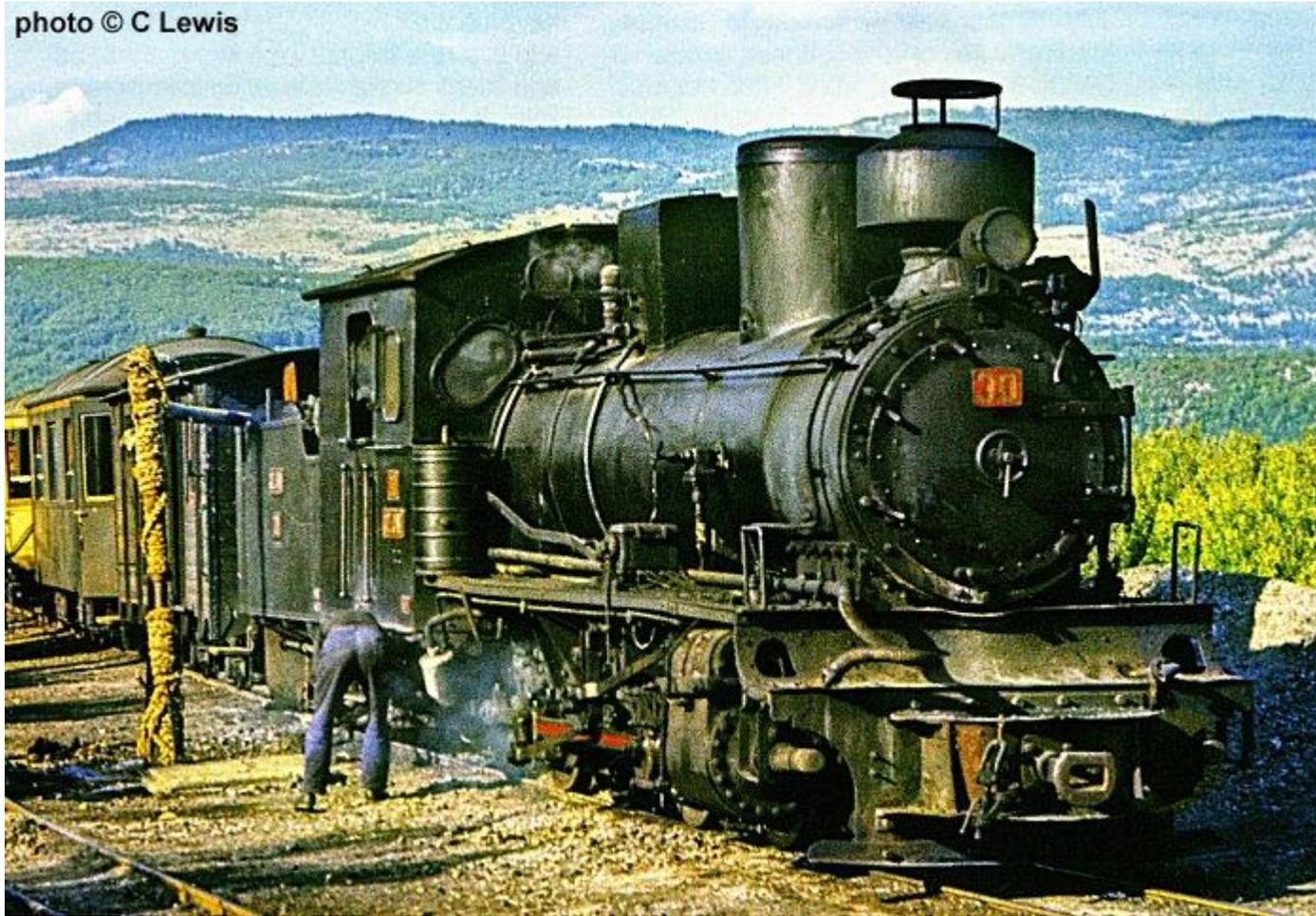
**The train from Drvar to Licka Kaldrma climbed out of the Unac valley for more than an hour before we stopped for water and fire cleaning at this remote spot. Steinbeisbahn No. 30 had been handling the load with ease. No. 30 was one of a series of four 0-10-0's Nos. 29 to 32 built by Orenstein & Koppel.**
