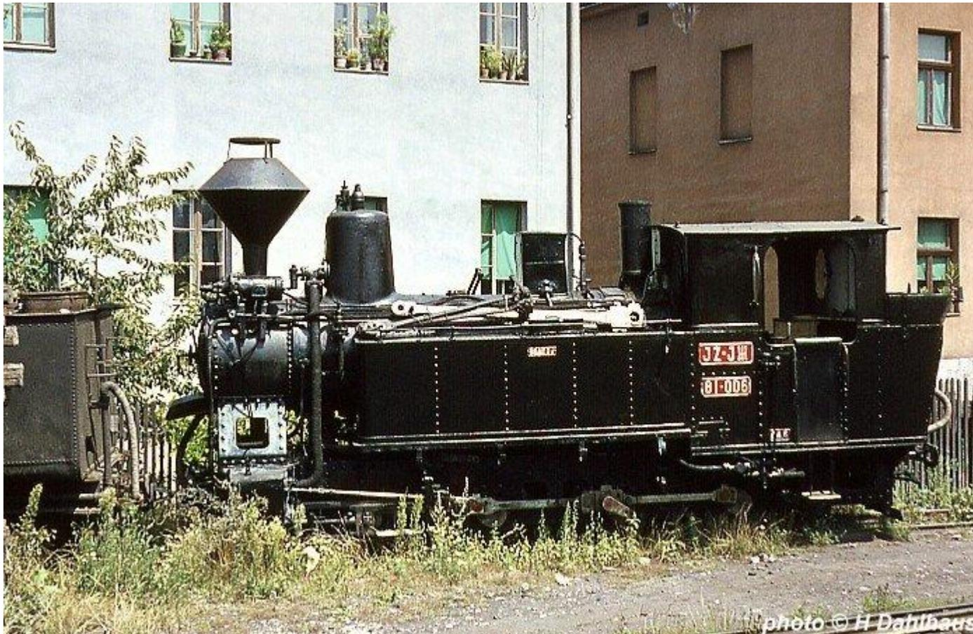
**Newly overhauled 81-006, an 0-8-0 tank built in Budapest in 1914, waits to return to its home depot of Zavidovici. This loco was built with Klien Lindner axles and was identical to the Budapest/MAVAG type 70 which was built between 1905 and 1950. A total of 142 were built and they were also found in Romania. 11th August 1966.**
