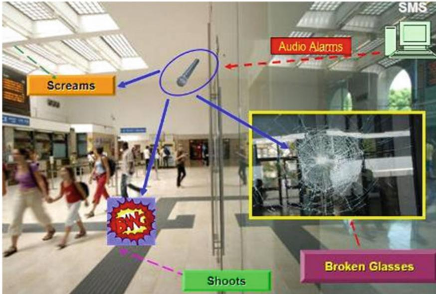
**Fig. 3** Events detected by an ASD system
