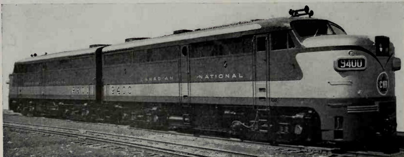
Canadian National Nos. 9400 & 9401, Class W-1-A; Two Unit 3,000-hp. Freight Locomotive built by Montreal Locomotive Works Ltd.—
