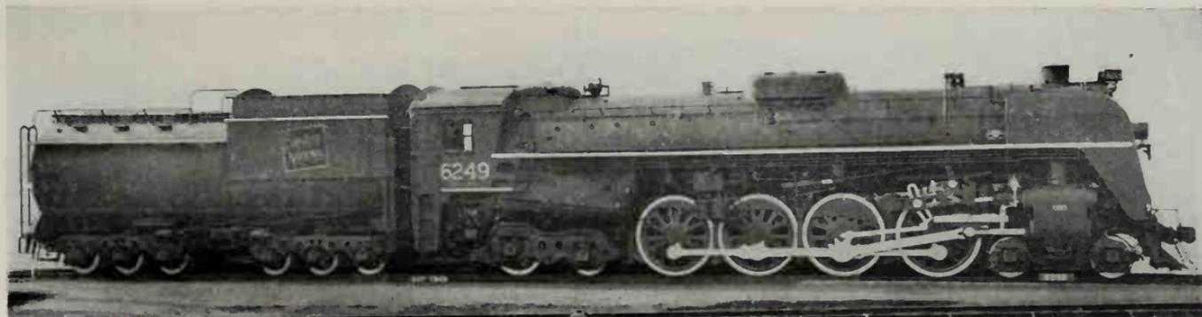
Canadian National 4-8-4 Type locomotive for passenger and fast freight service, Class U-2h, Nos. 6235-6264. Built by the Montreal Locomotive Works in 1943 and 1944.
