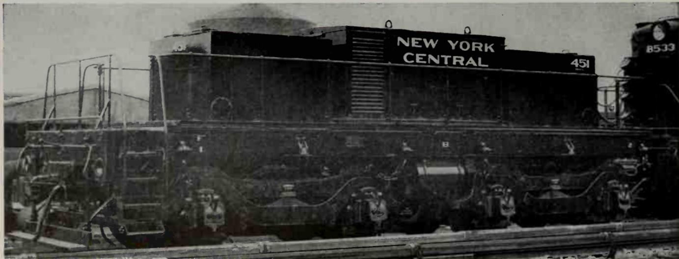
**New York Central Electric Auxiliary for Diesel Pushers, Class DHT-1a, operates an current drawn from Diesel-Electric Switchers.**
