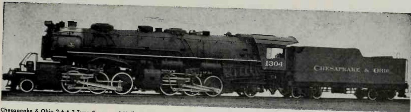
Chesapeake & Ohio 2-6-6-2 Type Compound Mallet Articulated Locomotive, Class H-6, Nos. 1300-1309. Built by The Baldwin Locomotive Works in 1949.
