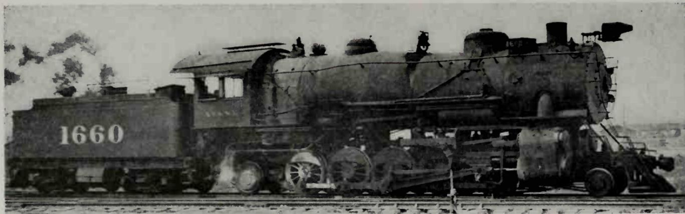
Atchison, Topeka & Santa Fe 2-10-2 (Santa Fe) Type Locomotive for heavy pushing and freight service. Built by The Baldwin Locomotive Works in 1907 and rebuilt at San Bernardino Shops in 1918.
