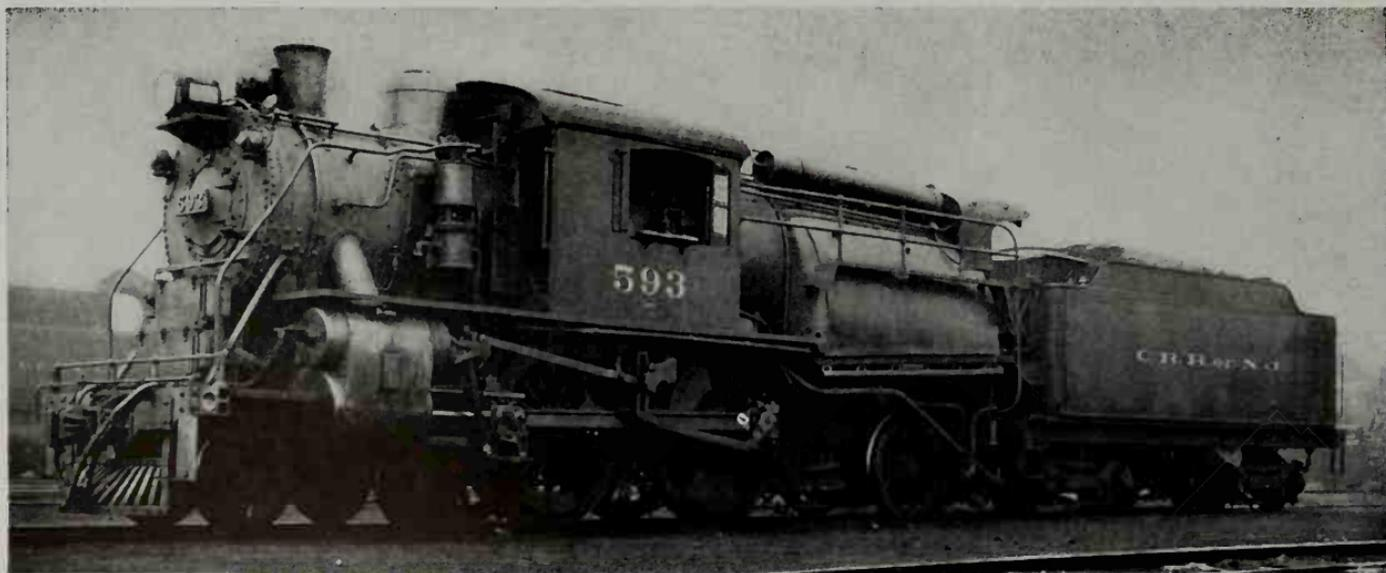
Central Railroad of New Jersey 4-4-2 (Atlantic) Type Locomotive, Class P-6, No. 593. Fast passenger locomotive built by the Brooks Works of the American Locomotive Co. in June 1902.
