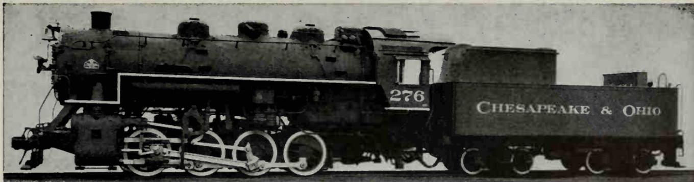
Chesapeake & Ohio 0-8-0 (Eight-Wheel) Switching Locomotive, Class C-16, Nos. 255-284. Built by The Baldwin Locomotive Works in 1948.
