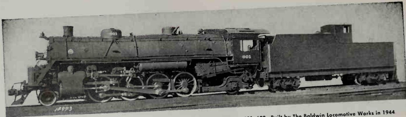
Kansas, Oklahoma & Gulf 2-8-2 (Mikado) Type Locomotive for freight service, Nos. 601, 602. Built by The Baldwin Locomotive Works in 1944
