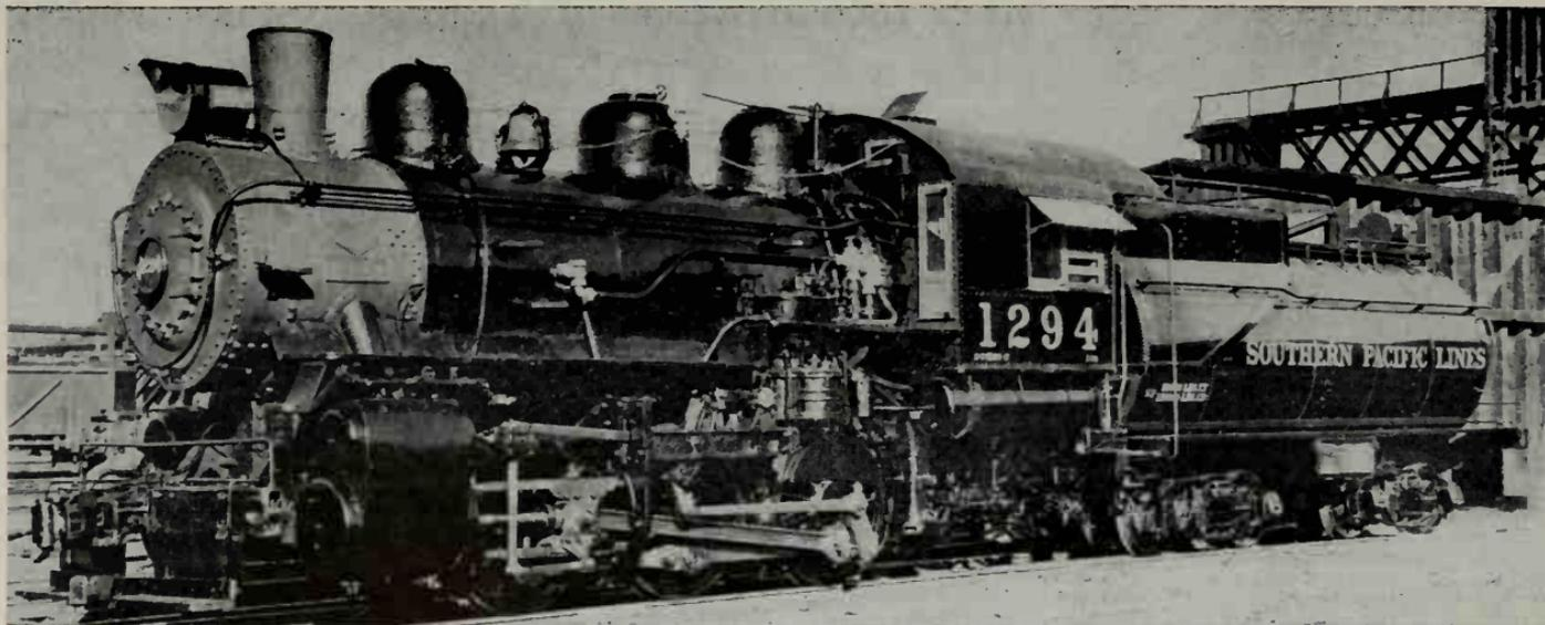
Southern Pacific 0-6-0 (Six-Wheel) Switching Locomotive, Class S-14, Nos. 1285-1294. Built by the Lima Locomotive Works, Inc., in 1924.
