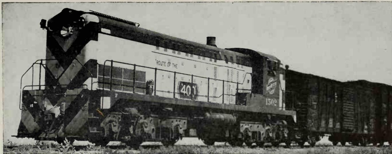
Chicago & North Western No. 1502, Baldwin-Westinghouse 1,600-hp. All-Service Locomotive with six axles and six motors, Model AS-616.
