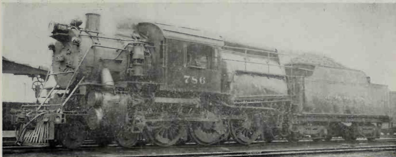
Central Railroad of New Jersey 4-6-0 (Ten-Wheel) Locomotive, Road Class L-8-s, later reclassified T-40, Nos. 780-789. Built by The Baldwin Locomotive Works in 1918.
