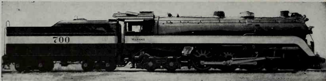
Wabash 4-6-4 Type Locomotive, Class P-1, Nos. 700-706. Rebuilt by the road from 2-8-2 Type Locomotives in 1943.
