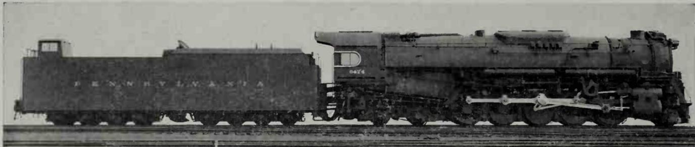
Pennsylvania Railroad 2-10-4 Type Locomotive, Class J-1, No. 6474. Built by the Pennsylvania Railroad Company in 1942, 1943 and 1944.
