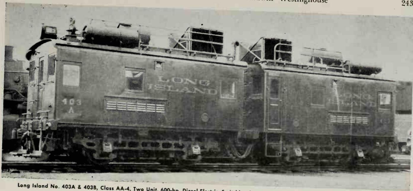
Long Island No. 403A & 403B, Class AA-4, Two Unit, 600-hp. Diesel-Electric Switching Locomotive built by The Baldwin Locomotive Works—
