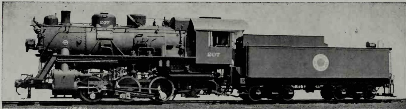
Lehigh & New England 0-6-0 (Six-Wheel) Switching Locomotive, Class B-5, No. 207. Built by The Baldwin Locomotive Works in 1936.
