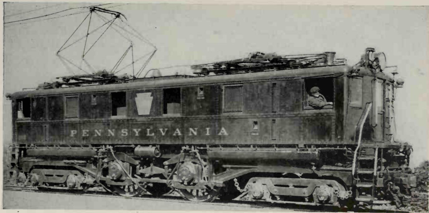
Pennsylvania Railroad 11,000-volt Alternating Current Locomotive, No. 7850, Class O-1, for passenger service, built at Altoona in 1930.
