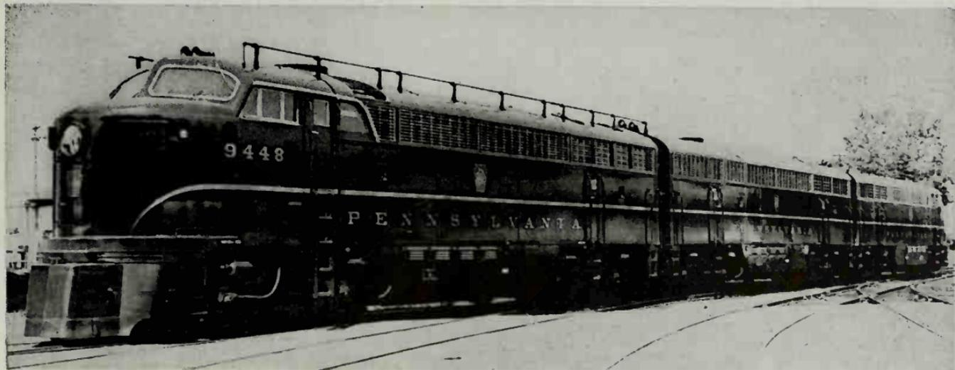
Pennsylvania No. 9448, Class FF-16, Three Unit, 4,800-hp. Freight Locomotive built by Fairbanks-Morse & Company in 1950.
