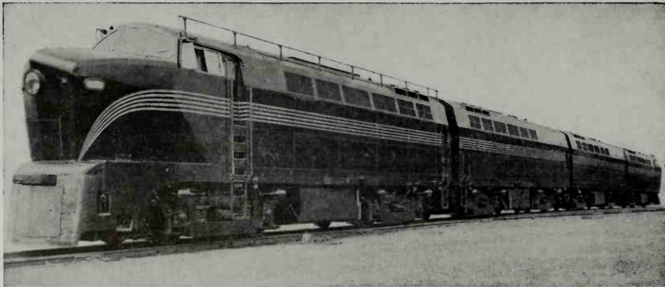
Baldwin-Westinghouse 6,400-hp. Locomotive with four RF-16 units.
