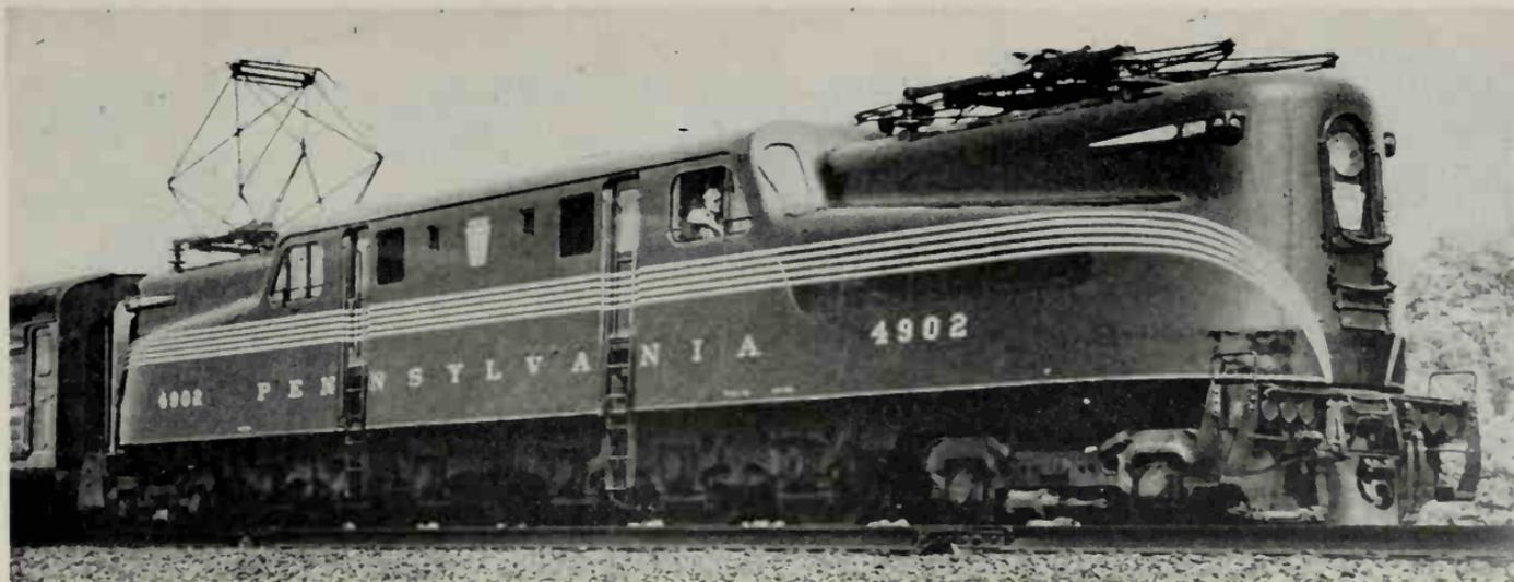
Pennsylvania Railroad 11,000-Volt Alternating Current Locomotive, Class GG-1, Nos. 4800-4938, for passenger service, built by General Electric Company, Westinghouse Electric Corporation, The Baldwin Locomotive Works and Pennsylvania Railroad.
