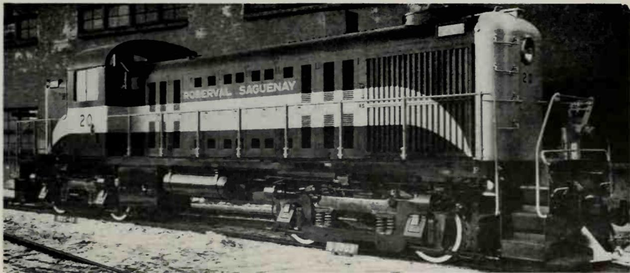
Roberval Saguenay No. 20, 1,500-hp. Road Switching Locomotive built by Montreal Locomotive Works Ltd.-Canadian General Electric Company Ltd. in December 1949.
