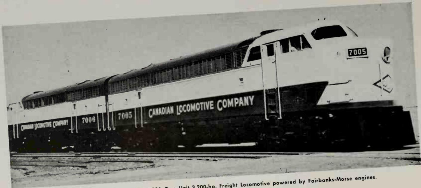
Canadian Locomotive Company, Ltd. No. 7005 & 7006, Two Unit 3,200-hp. Freight Locomotive powered by Fairbanks-Morse engines.
