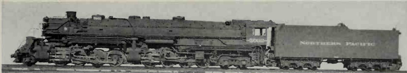
Northern Pacific 2-8-8-4 (Yellowstone) Type Locomotive, Class Z-5, Nos. 5001-5011. Built by The Baldwin Locomotive Works in 1930.
