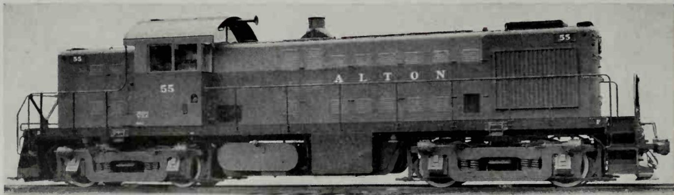
Alton No. 55, Class DSA; 1,000-Hp. Road Switching Locomotive built by American Locomotive Company-General Electric Company in Nov. 1945.
