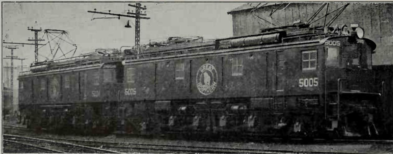
Great Northern Double-Unit Motor-Generator Type Electric Passenger and Freight Locomotive, Class Z-1, built by The Baldwin Locomotive Works and Westinghouse Electric Corporation in 1926.
