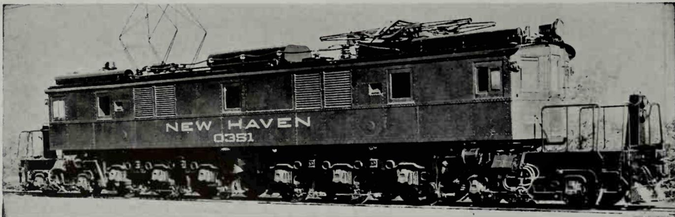
New York, New Haven & Hartford 11,000-volt A.C. and 600-volt D.C. Electric Passenger Locomotive, Class EP-3, Road Nos. 0351-0360, built by Westinghouse Electric Corporation and The Baldwin Locomotive Works in 1931.
