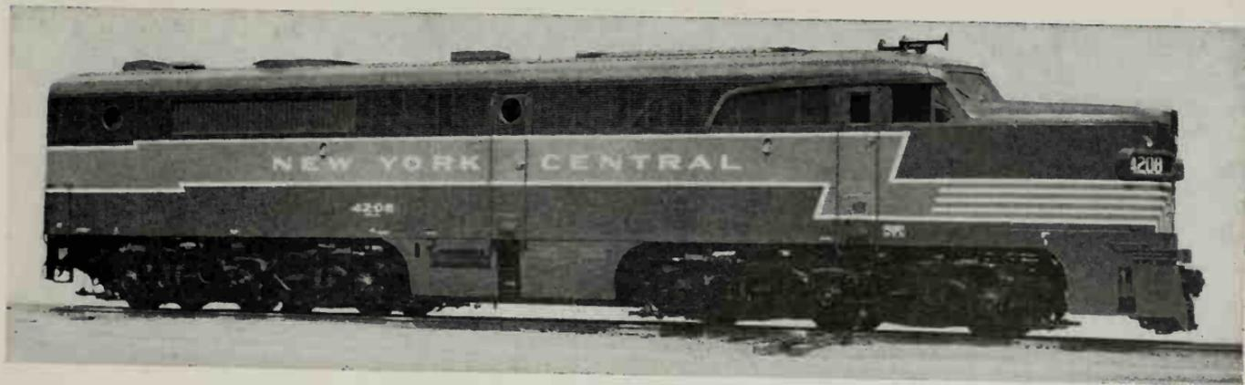
New York Central No. 4208, Class DPA-4a; 2,250-Hp. Passenger Locomotive built by American Locomotive Company-General Electric Company in June 1950.
