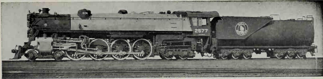
Great Northern 4-8-4 Type Locomotive, for passenger service, Class S-2, Nos. 2575-2588. Built by The Baldwin Locomotive Works in 1930.
