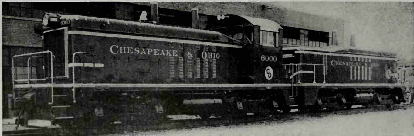
Chesapeake &amp; Ohio No. 6000, Two Unit 2,400-hp. Transfer Locomotive.
