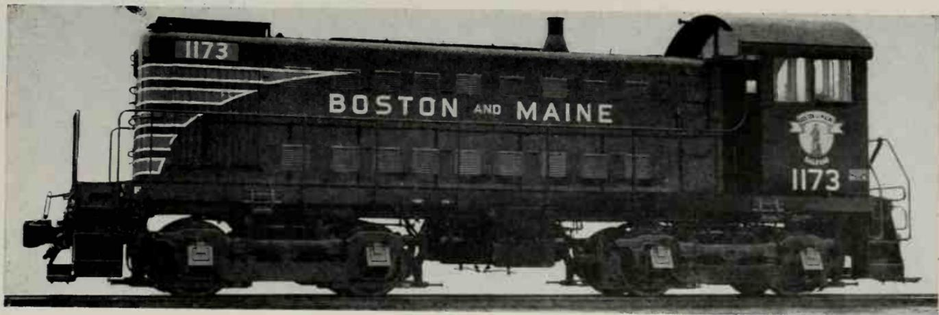
Boston & Maine No. 1173; 660 Hp. Switching Locomotive built by Alco-G.E. in September 1950.
