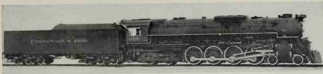
Chesapeake & Ohio 4-8-4 Type Locomotive for passenger service, Class J-3a, Nos. 605-606 and 610-614. Built by Lima Locomotive Works, Inc. in 1948.
