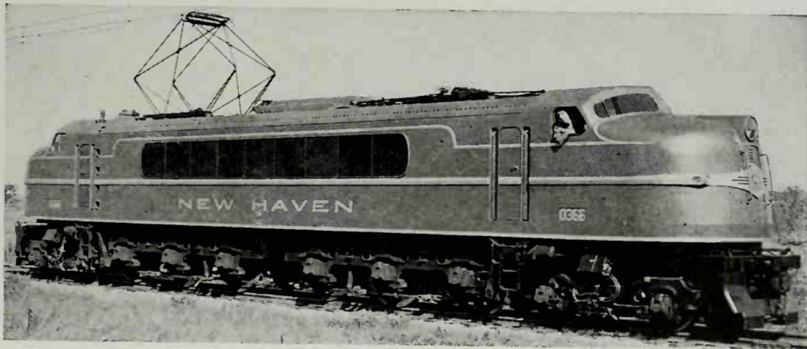
New York, New Haven & Hartford Electric Passenger Locomotive, Class EP-4, Road Nos. 0361-0366, combination 11,000-volt A.C. overhead and 600-volt D.C. third rail, built by General Electric Co. in 1938.
