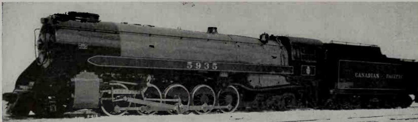
Canadian Pacific 2-10-4 Type Locomotive, Class T-1c, No. 5935, for freight service, Nos. 5930-5935. Equipped with Booster. Built by the Montreal Locomotive Works, Ltd. in 1949.
