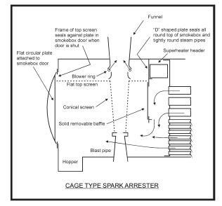
My experience has been that if the screen area is made too large or there is insufficient draught it will block up with soot and if it is made too small it will block up with cinders. Screen holes are made with a punch which leaves a slightly tapered hole. The side where the punch enters is smooth, with rounded edges, and the side where the piece is punched out is rough. It was important to place the rough side towards the fire.
