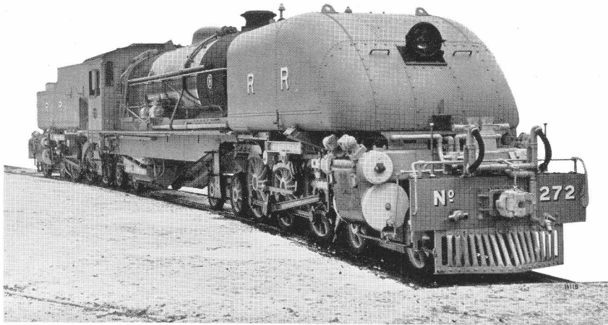
Rhodesia Railways. 3 ft. 6 in. Gauge. 4-6-4+4-6-4 Passenger Type "Beyer-Garratt" Locomotive for 60 lb. Rail. Built by Beyer, Peacock and Co. Ltd., and fitted with "MeLeSco" Superheater.
