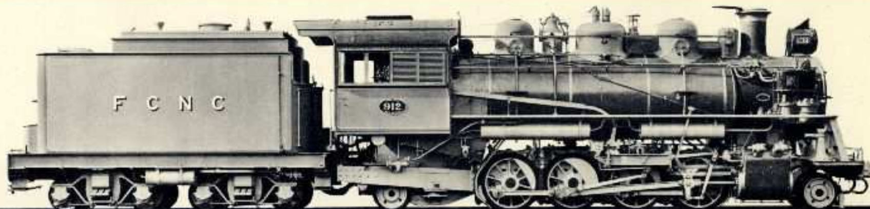
ANTOFAGASTA (CHILI) & BOLIVIA RAILWAY TYPE 2-8-2 SERVICE — GENERAL PURPOSE No. 153
