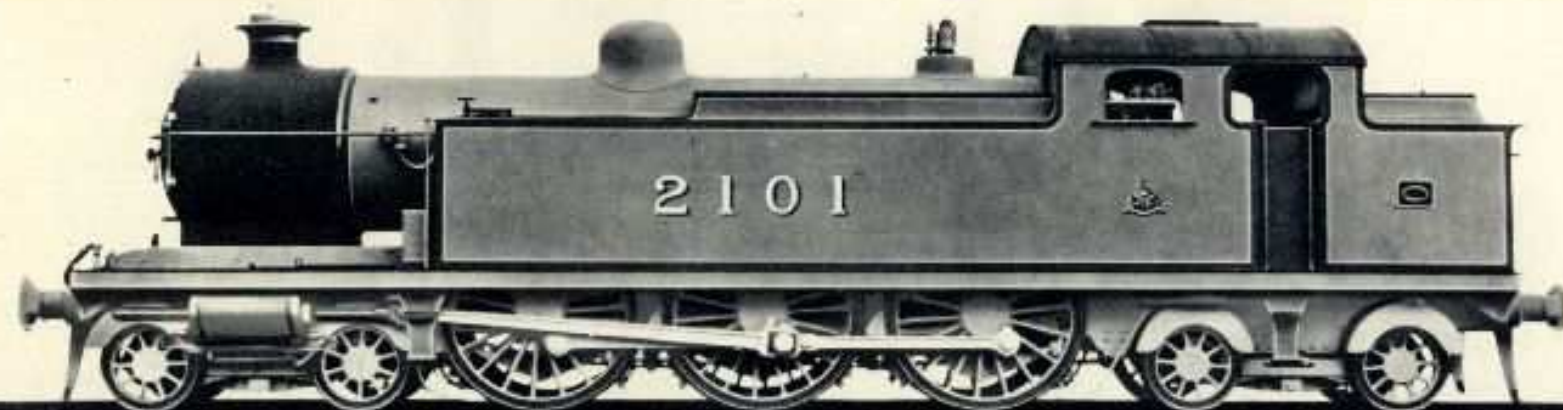
LONDON, TILBURY AND SOUTHEND RAILWAY TYPE 4-6-4T SERVICE — EXPRESS PASSENGER No. 0396
