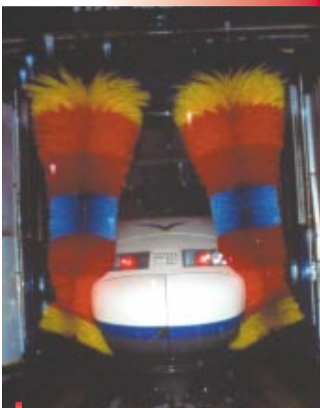
Train washing at AVE maintenance depot
