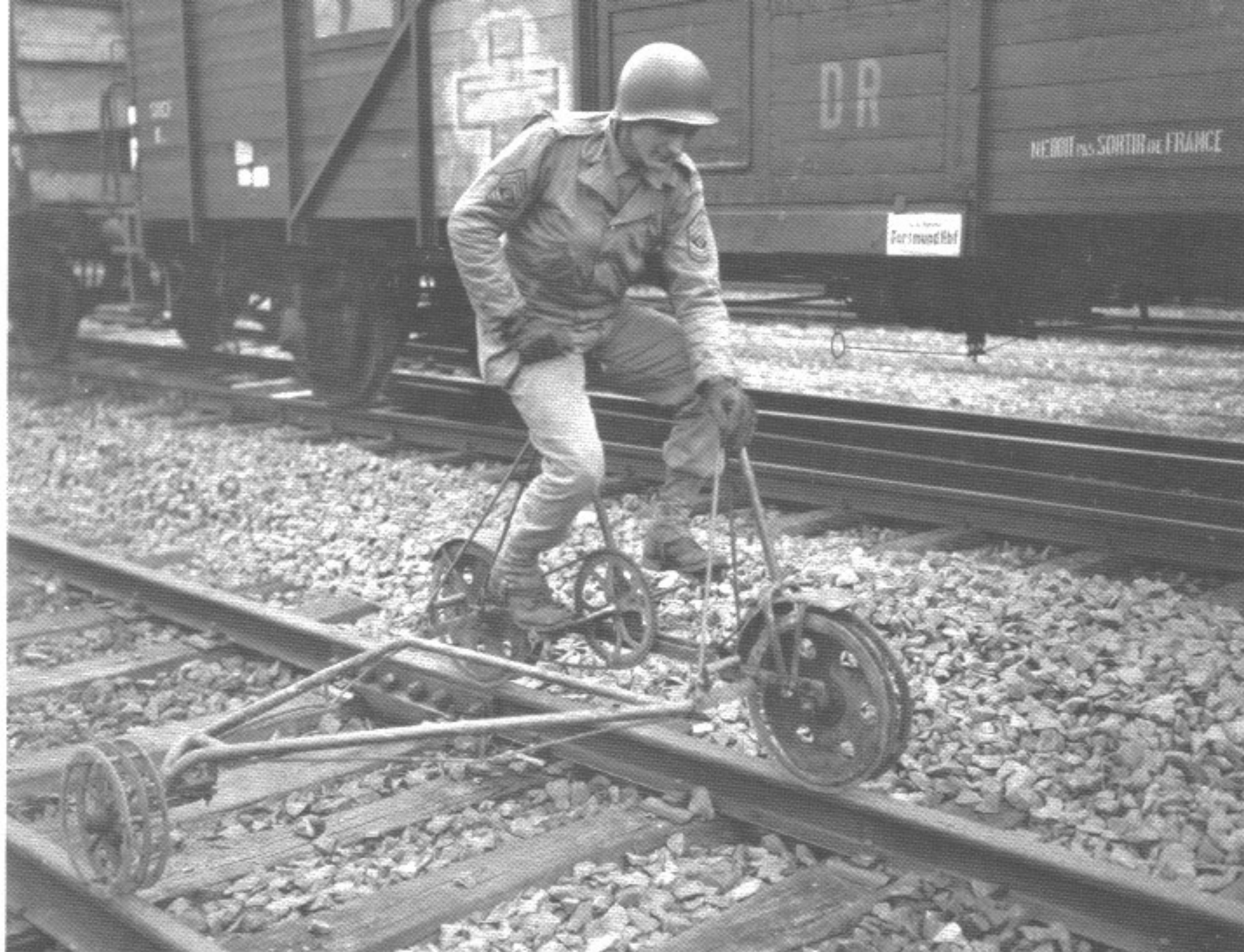
In Bendorf, France, 1st Sgt. Herman Warner, Sacramento, CA, is photographed riding the vehicle which was used to test track gauge after repair. (12-3-44)
