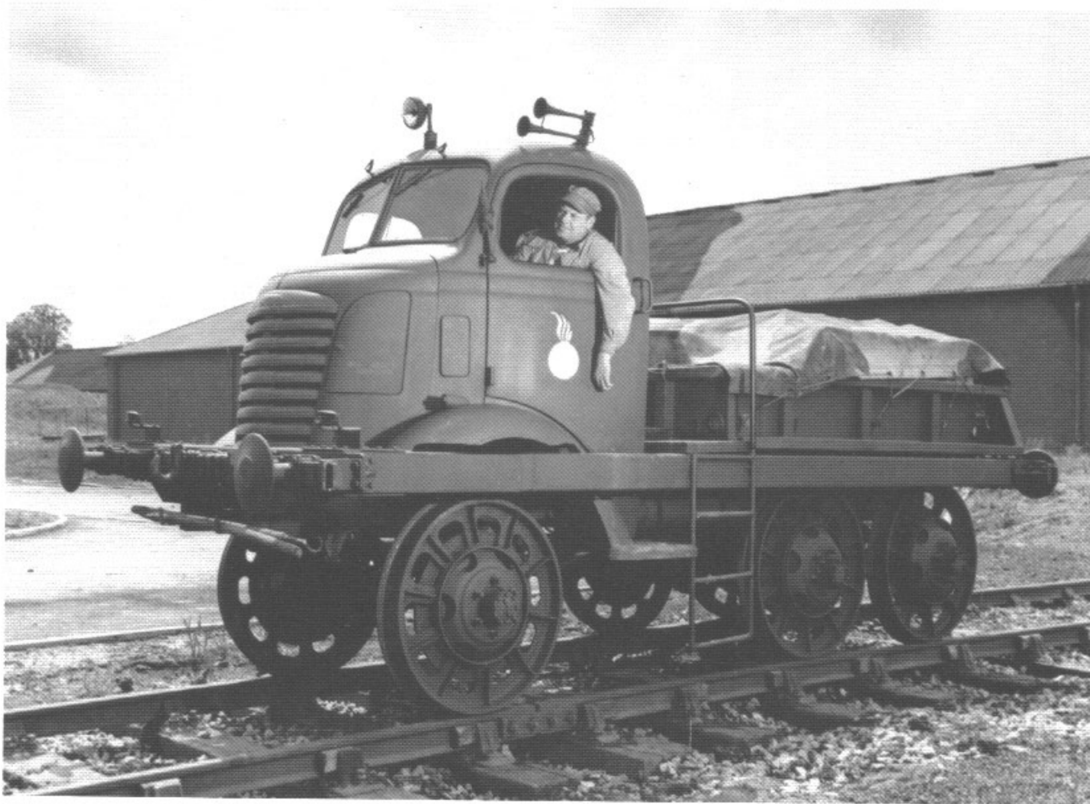
At Ashchurch, England, Cpl. "Big John" Baraniak, Port Ready, NY, engineers this switch engine made from a GMC truck. (6-16-43)
