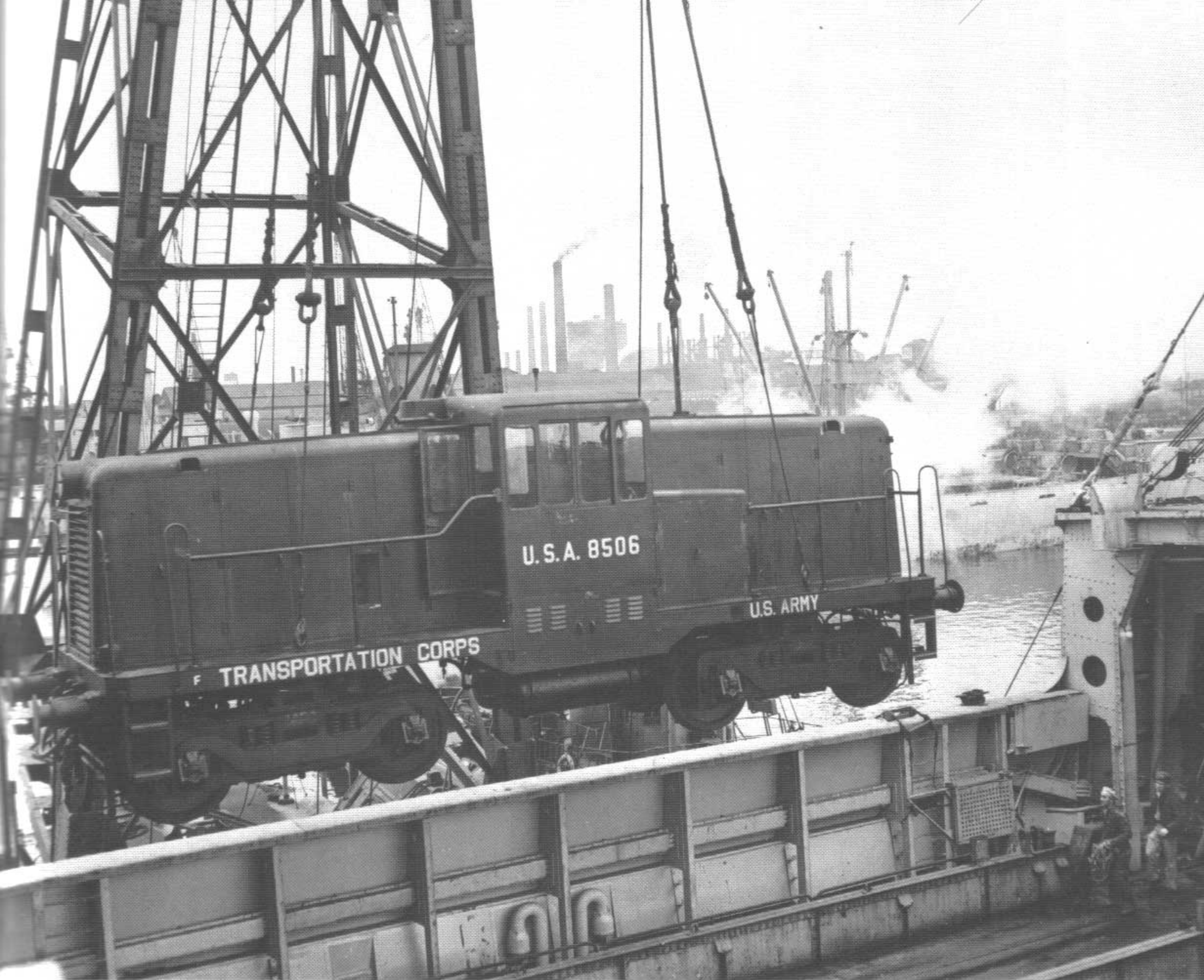
A diesel is loaded in an English port for Channel crossing to France. Transportation Corps personnel conditioned these locomotives in English-loaned shops in Britain. (9-10-44)
