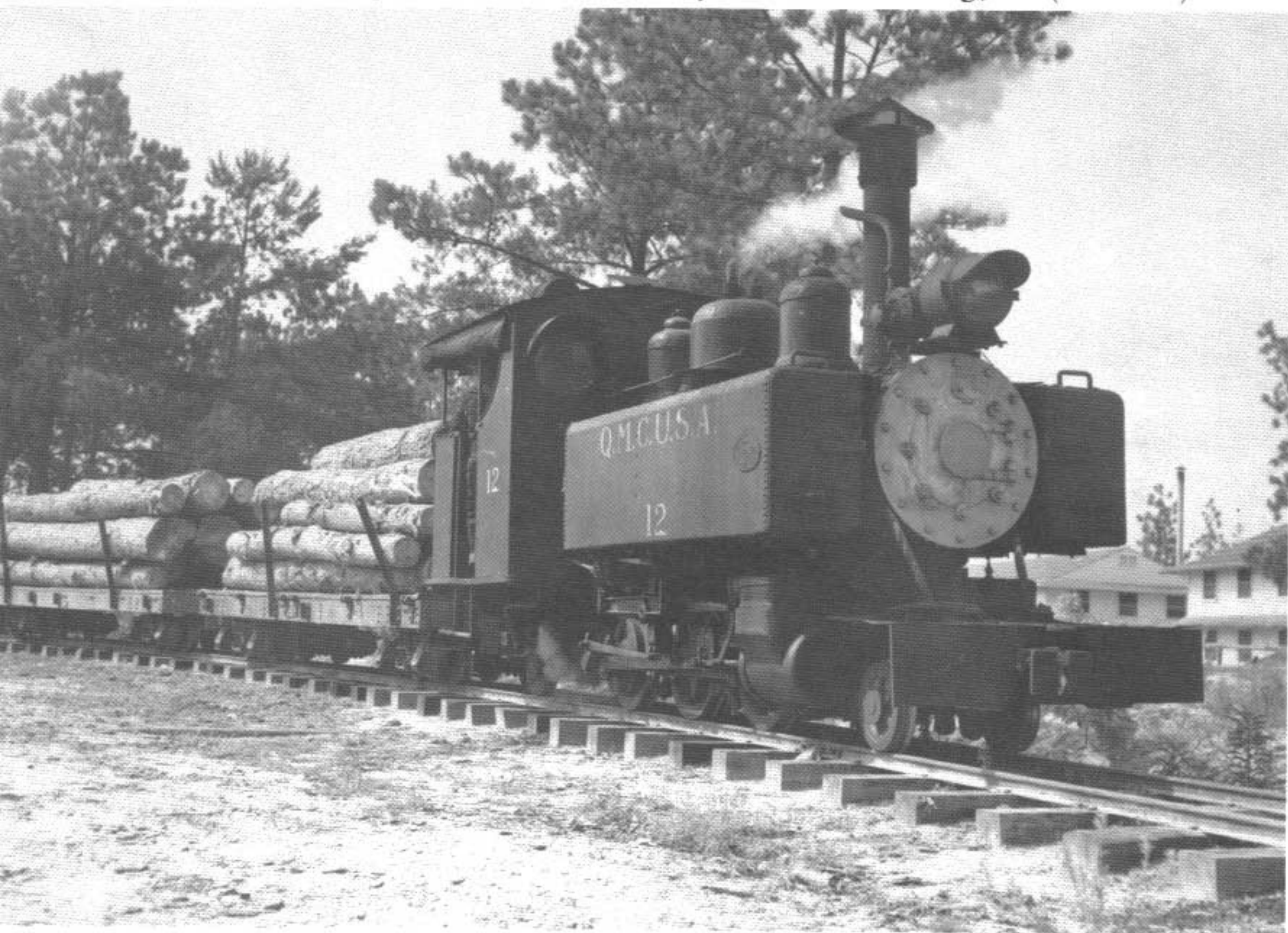
A Davenport narrow-gauge locomotive at Fort Benning, GA, pulls a train loaded with logs to a sawmill. (6-26-42)
