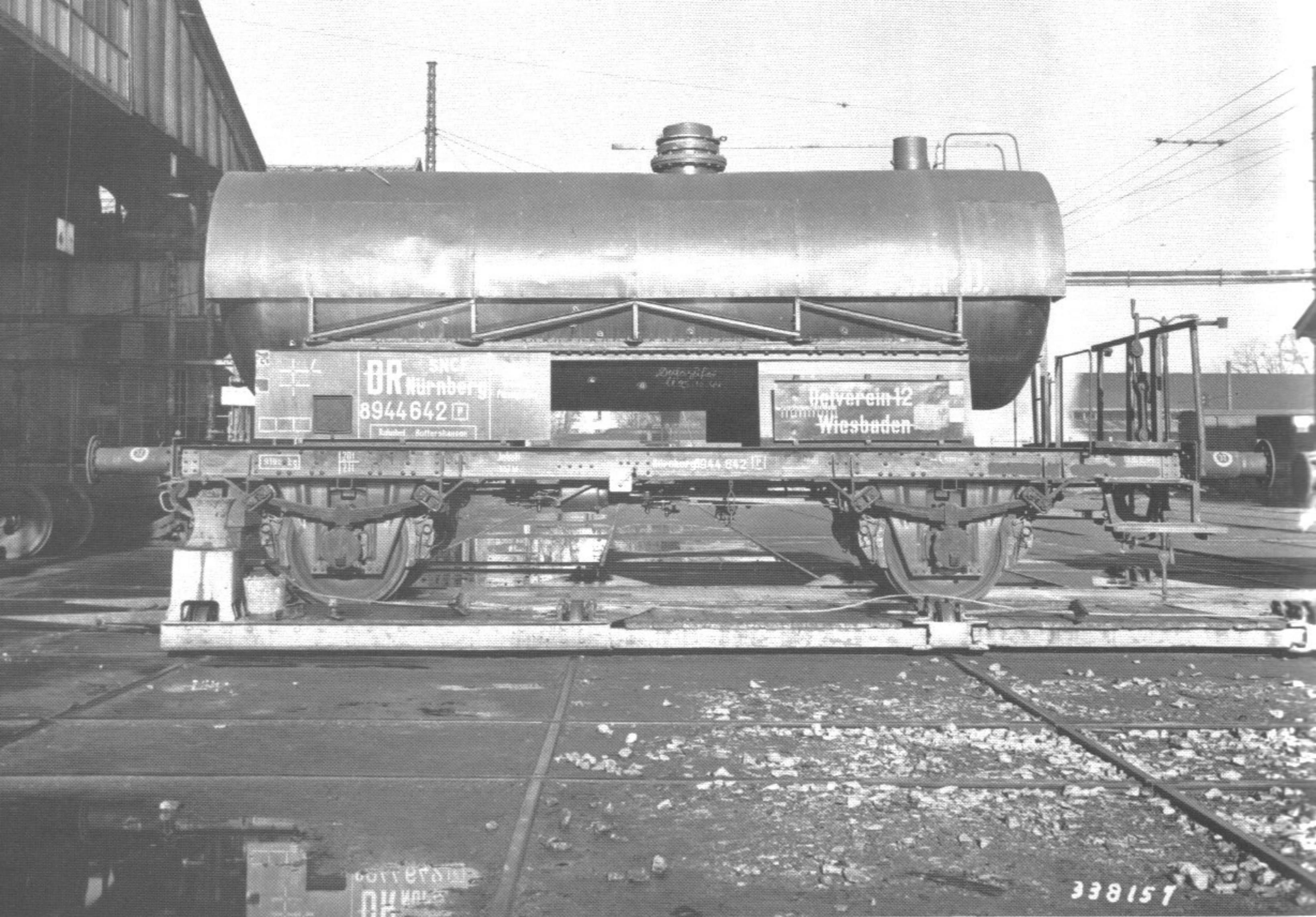
Photographed at the Brittany Base Section, Rennes, France, this captured German tank car was believed to have been used to carry hydrogen peroxide, “a liquid explosive for the robot bomb,” better known as the V-2 rocket. (12-11-44)
