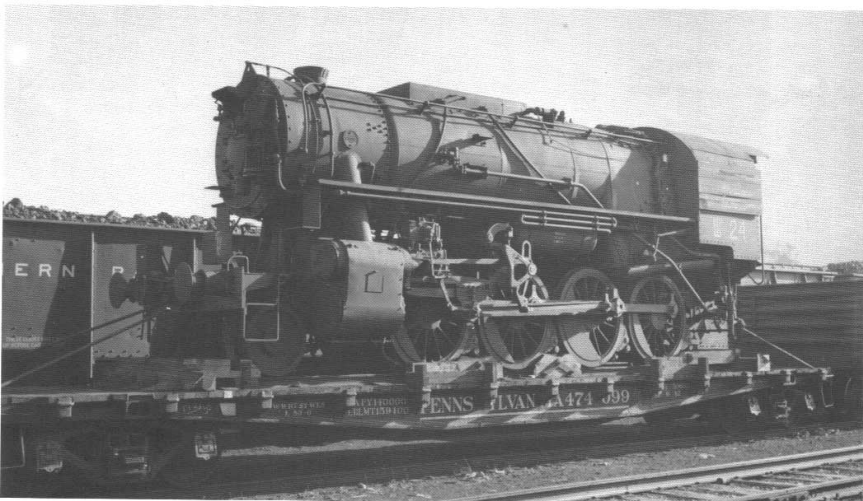
An American-built locomotive is moved on a flat car because the track gauge of Russian railroads is wider than that in the U.S.
