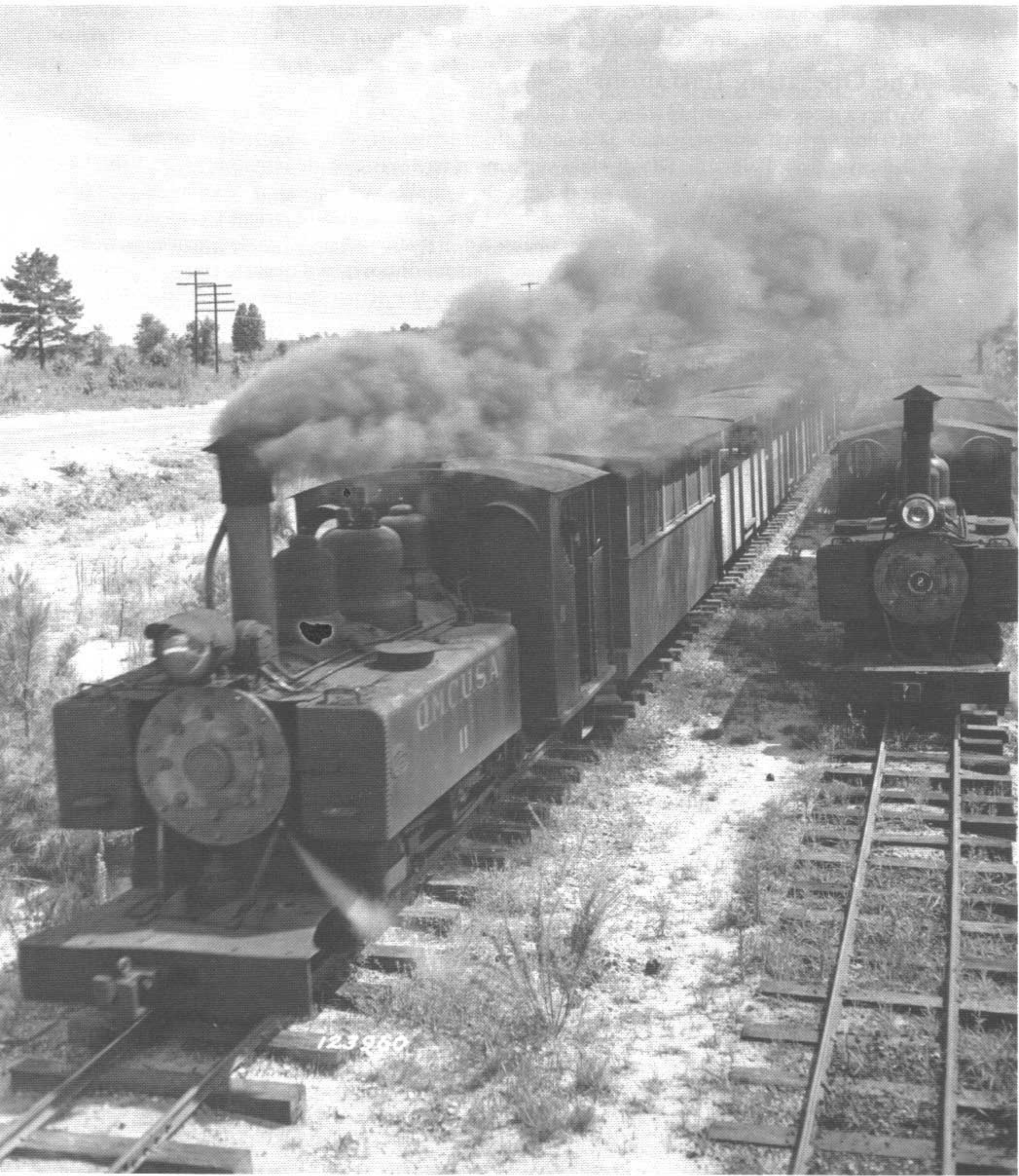
Narrow-gauge locomotives used to transport troops at Langley Ridge, Fort Benning, GA. (7-28-41)
