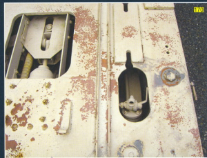
169 170 More views of the brake cylinder. One of the angle cocks for the steam hoses can be seen in the bottom right.
