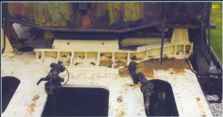
1433 1434 2006 The front of the traversing mechanism. Note the sliding cover for the operating shaft.
