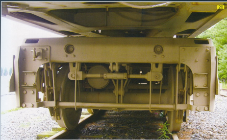
20 View of the railway truck from underneath the gondola. Its bottom can just be seen in the top of the picture. To the left and right are the hangers for the brake shoes. They are joined at the bottom to a rod that connects to the central brake mechanism seen in the middle. On the top left is a hook for attachment of the chain connecting the railway truck and the gondola in transport. This chain would have prevented the railway truck from shearing when derailling. Keeping the trucks in a straight line would minimize damage in case of accidents. Bear in mind that K5's were able to use bad or quickly laid temporary track, so accidents were taken into account.
