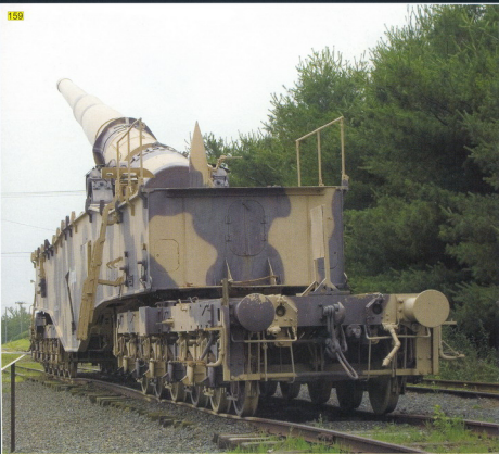
168 Overall view of the rear of the gun. The ladder extends quite far from the side of the gondola. The ladder consists of three parts that can slide up to shorten it. The outrigger can be collapsed and the whole assembly stowed on the side of the gondola with two hooks seen in the picture.
