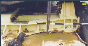
2006 The back of the traversing mechanism. The switchbox in the middle has retained both its arms. On the ends of the slide are metal bars that activate the switches; the one on the right is missing.
