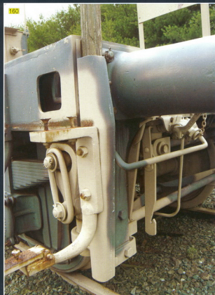
169 The side of the coupling, showing the draft hook.
