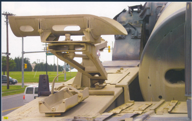
653 A good view of the cartridge catcher. The stand for the rammer should be behind it. This rammer was used to release the breechblock when it became jammed. The container in front is for stowing it (see photo [171]).
