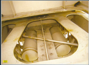
21 22 23 Several views of the pressure vessels for the brakes. The pressure drives central brake cylinders that operate the brakes through a system of rods and hangers.
