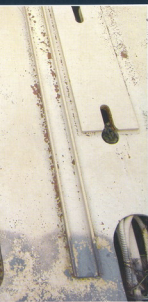
167 The top of the rear railway truck. The rails for the generator run along it. The rectangular plates with keyhole slots play a role in fastening the generator to the railway truck. Triangular structures were attached here to which the generator truck was fastened (see photo [212]). The hole in the middle shows one of the brake cylinders.
