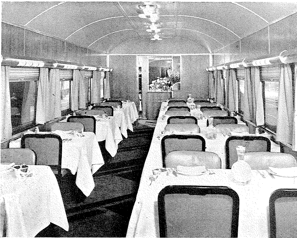
The Dining Car at Night—The Lighting Includes Both Center and Side Fixtures
